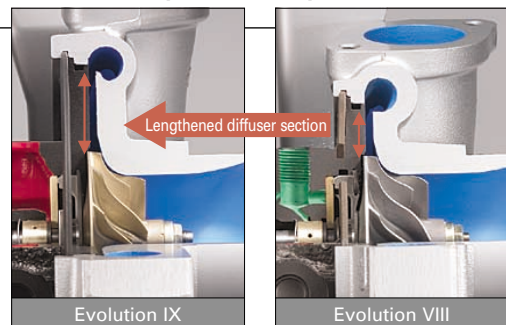
Increasing the diffuser section length improves response at low- to mid-range speeds
