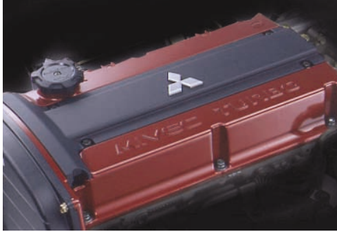
2.0-liter 16-valve DOHC MIVEC with intercooled turbocharged
